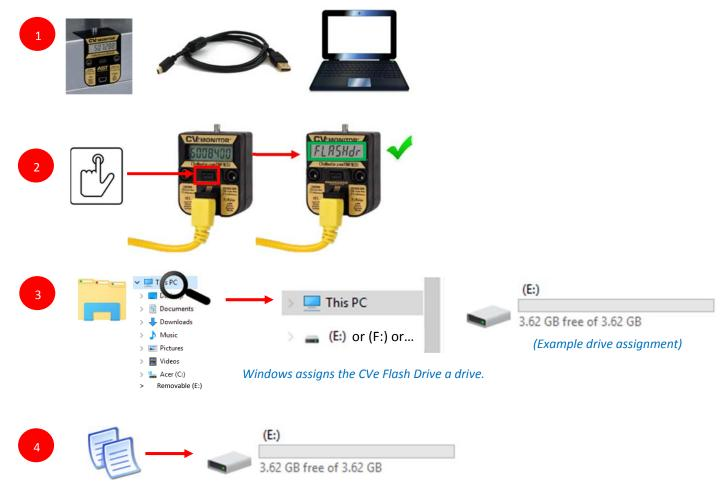
Copy desired files to the assigned drive. These files stay on the CVe Monitor Flash Drive.
